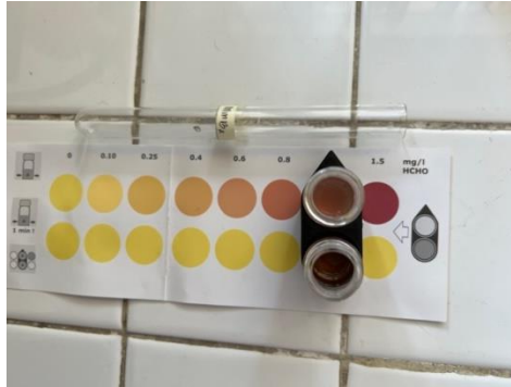
2-An example measurement reading of positive sample of sausage
