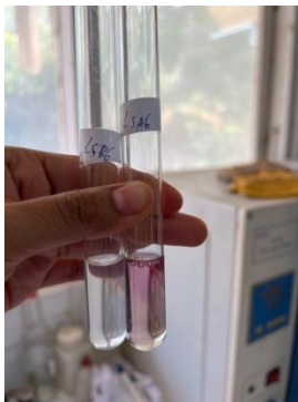
3-An example of frozen chicken sample positive of formalin contamination
