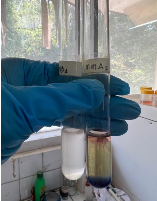
Figure 8. Pork sausage positive of formadehyde at the level of 9 mg/kg
