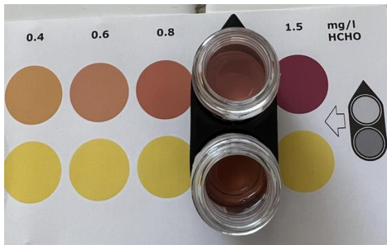
6- An example measurement reading of formalin positive sample of frozen fish
