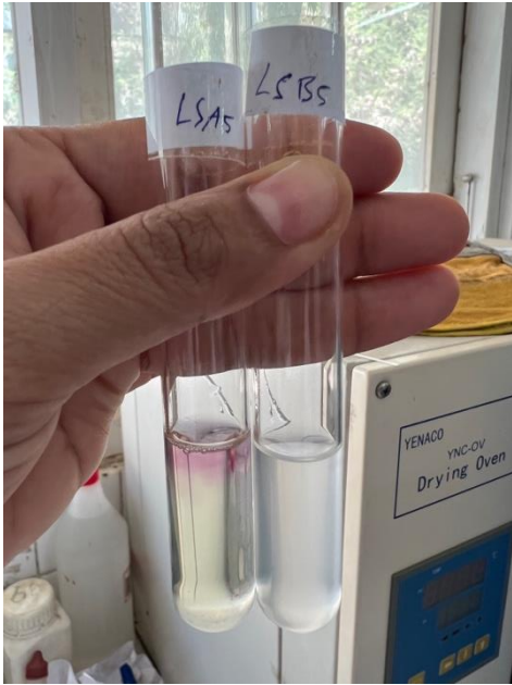
Figure 6. Whole chicken sample positive of formalin at the level of 9 mg/kg
