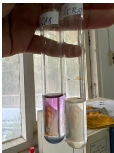
5- An example of fish sample positive of formalin contamination
